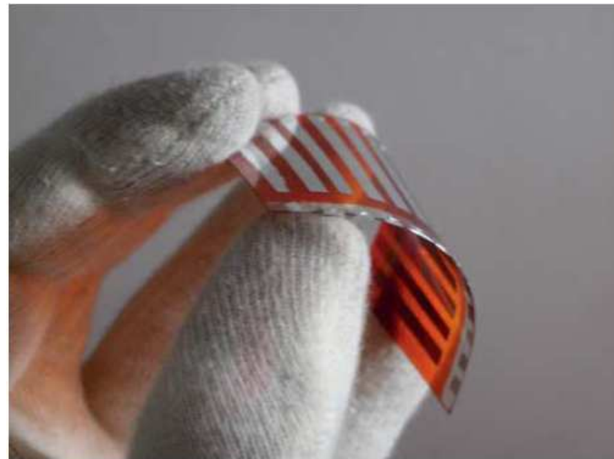
MDMO-PPV:PCBM solar cell realized on a PET substrate
